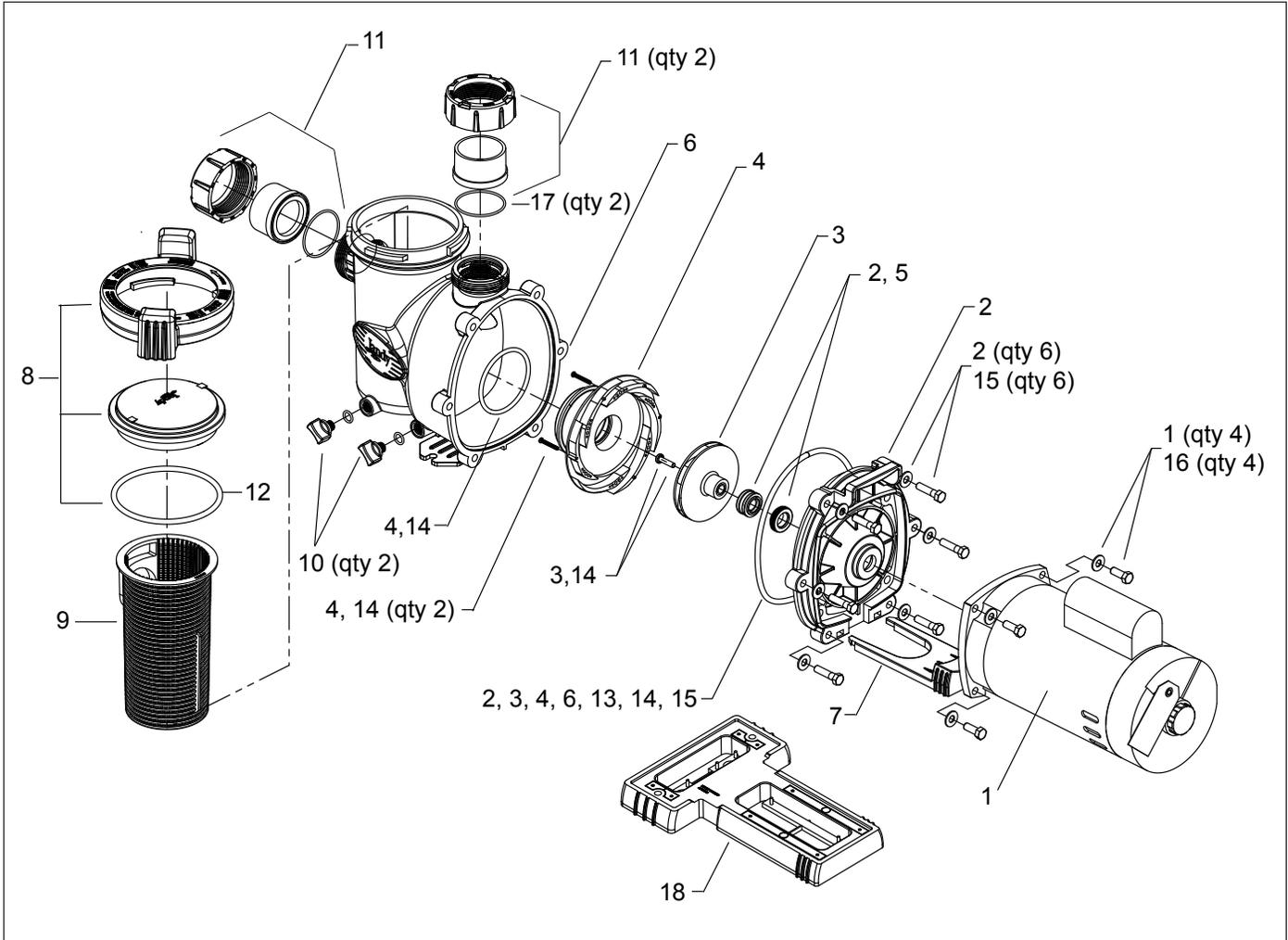
Figure 15. FHP Exploded View
